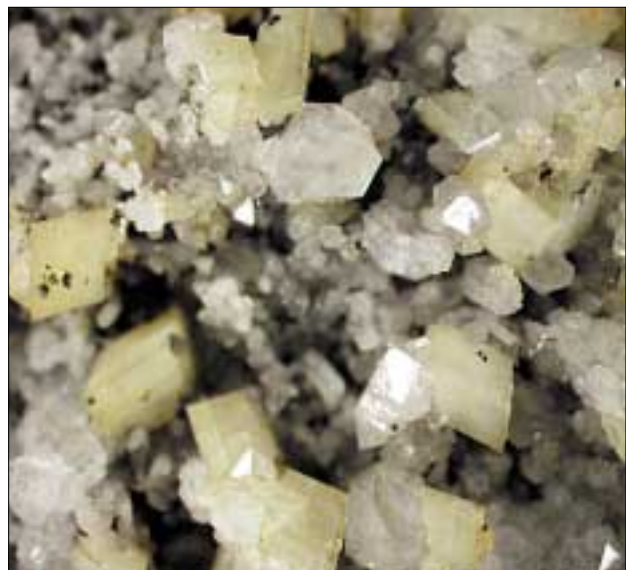
Figure 16. Mineralised fracture in coal strata from Nant Helen open pit in the South Wales Coalfield. Minerals shown are quartz (pyramidal crystals), Ankerite (rhombic crystals) and Chalcopyrite (small dark crystals overgrowing the ankerite) (courtesy of University of Cardiff)
